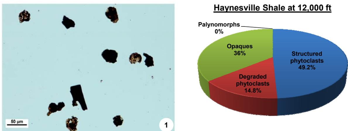
**Fig. 1**-Percent distribution and photomicrograph of the kerogen components identified from Haynesville Shale which are dominantly phytoclasts and opaques.
