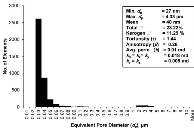
Fig. 12-Fayetteville Shale pore size histogram resulted from 3D pore model.
