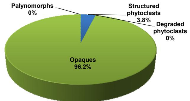
Fig. 3-Percent distribution and photomicrograph of the kerogen components identified from Utica Shale, Dolgeville member at the depth of 4,878 ft which are dominantly opaques.
