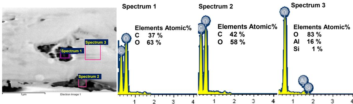
Fig. 9-EDS spectrum analysis of Fayetteville Shale at depth of 2,351 ft; spectrum 1 and 2 confirm kerogen presence, and spectrum 3 represents aluminum silicate (clay).
