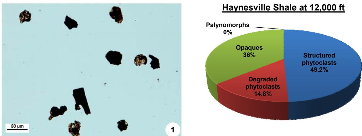
**Fig. 1**-Percent distribution and photomicrograph of the kerogen components identified from Haynesville Shale which are dominantly phytoclasts and opaques.
