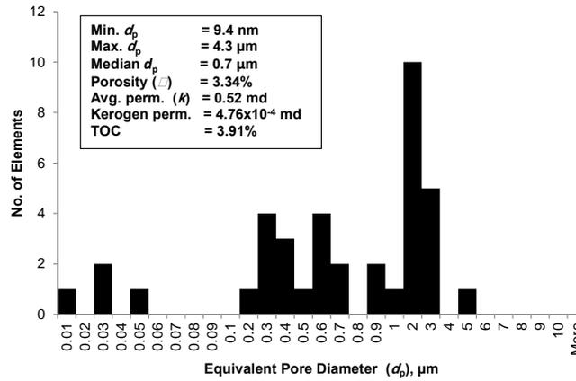
Fig. 10-Fayetteville Shale kerogen pore size histogram resulted from 2D pore model.
