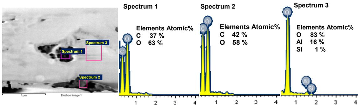
Fig. 9-EDS spectrum analysis of Fayetteville Shale at depth of 2,351 ft; spectrum 1 and 2 confirm kerogen presence, and spectrum 3 represents aluminum silicate (clay).
