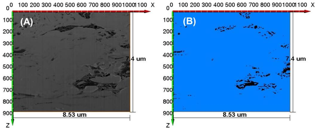
Fig. 8-2D kerogen pore model of Fayetteville Shale at depth of 2,351 ft; (A) SEM images showing the organic matter, and (B) Converted 2D binary image of 0 and 1 pixel values.
