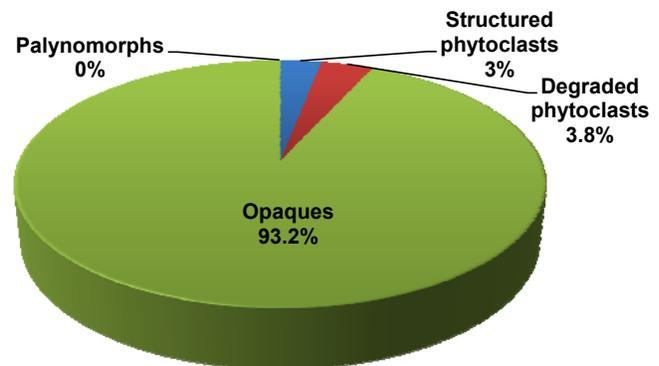
Fig. 5-Percent distribution and photomicrograph of the kerogen components identified from Fayetteville Shale which are dominantly opaques.
