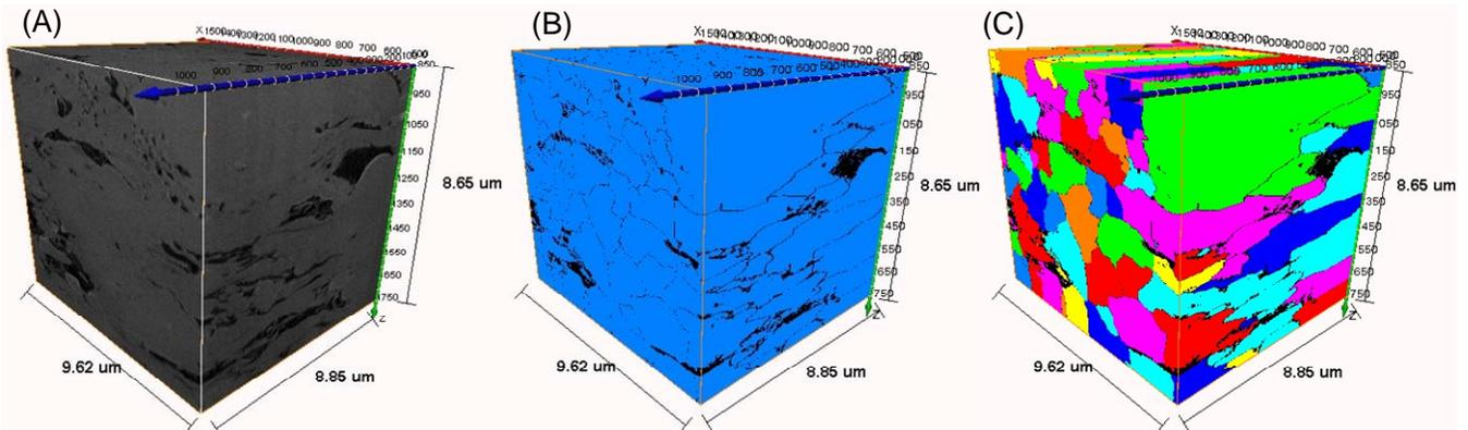
Fig. 11-3D pore model of Fayetteville Shale (A) 200 slices of 2D-SEM images are aligned and stacked, (B) Converted 3D stack to binary image of 0 and 1 voxel values, and (C) Element boundaries are determined and labeled to perform the porosimetry analysis.
