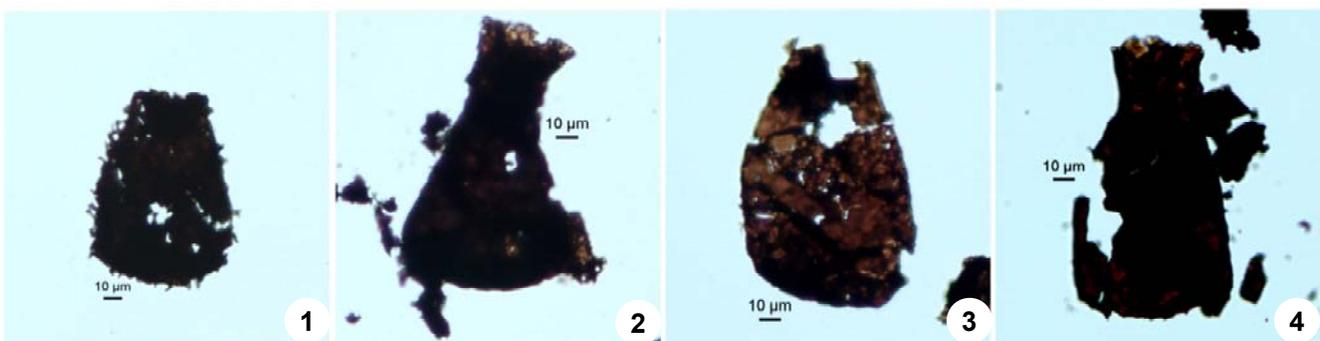
Fig. 6-Photomicrographs of some of the chitinozoan specimens identified from Utica and Haynesville shale-gas source rocks.
