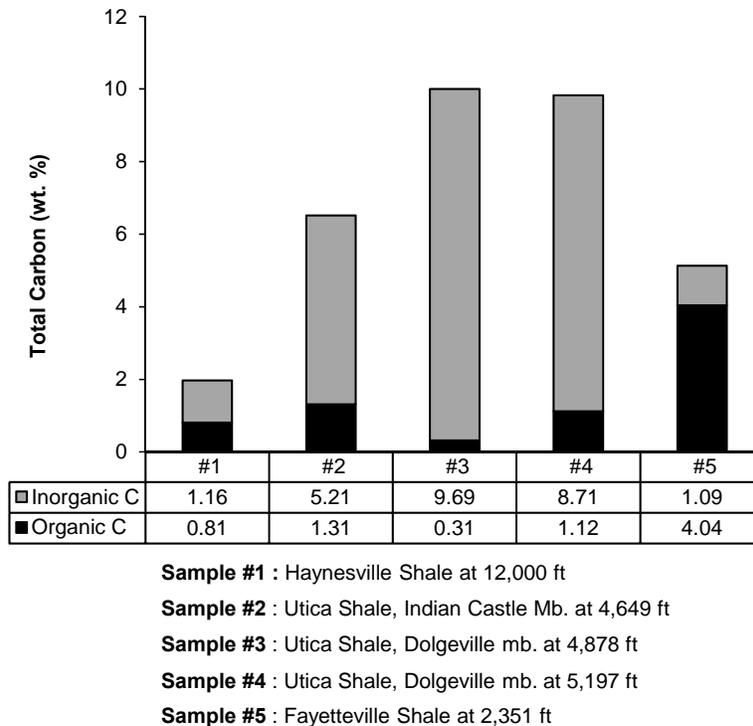
Fig. 7-Measured total carbon (inorganic and organic) from the studied shale-gas source rock samples.
